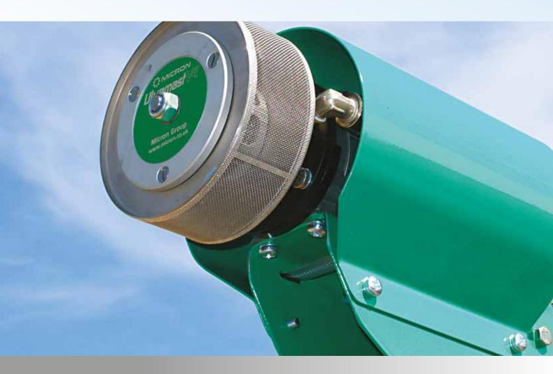
The Ulvamast V4 is a vehicle-mounted ultra low volume (ULV) sprayer for the control of migrant pests such as locusts, grasshoppers and armyworm at spray volumes of 0.5 - 3.0 litres per hectare.
