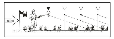
It is therefore <u>vital</u> to check the wind speed and direction before spraying. The diagrams below show acceptable wind direction and how the spray route should be planned:
