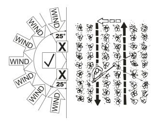
Best results will be obtained in a consistent crosswind of between 1 and 4 m/s. <u>Never</u> spray when there is no wind, or wind direction or speed is changeable, since the operator then risks being contaminated by the spray. <u>Always</u> hold the spray head at least one metre away from any part of the body to avoid the risk of direct contamination by the spray. <u>Never</u> touch the atomiser disc when it is spinning.
