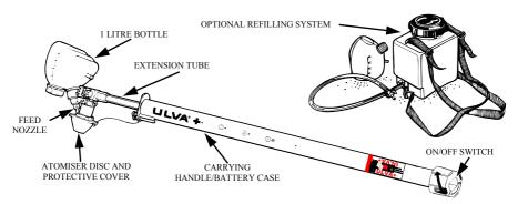
Specially designed *Micropak* backpacks can be supplied for use with the ULVA+, with a refilling system to refill the one litre spray bottle fitted to the spray head. Only use ULV formulations with a backpack if appropriate chemically resistant tubing is available (e.g. Micropaks fitted with EVA tubing).
