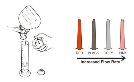
**Example:** Required spray volume = 10 l/ha; Spray pass interval = 3m Flow rate measured = 150 ml/min
