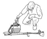
Half fill the tank with clean water. Check for leaks. Add the measured product.
