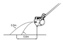
If the spray head is horizontal the spray will project ahead about 0.6 metres and spread 0.5 metres
