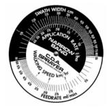
4. Having fixed the swath (band) width and application rate select the preferred walking speed (2km/hr = Slow, 3km/hr = Medium, 4 km/hr = Fast).
