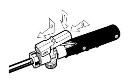
If the master electric switch is in the off position the dual control switch will regulate liquid flow only.
