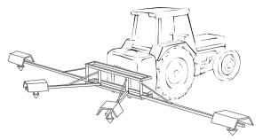
Figure 3 – A boom sprayer for orchard floors
