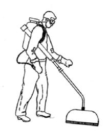
Start walking immediately spray liquid is emitted. When spraying, the spray head should be held as close to the ground or the top of the weed canopy as possible with the shroud at an angle of approx. 5 degrees to the horizontal. The leading edge of the fringe fitted to the shroud should be touching the ground or the top of the weed canopy. The shroud will be seen to rotate. It is important to rotate the shroud as much as possible in order for the inbuilt Weedswiper to take effect.
