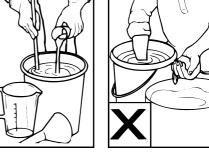
Always use the correct equipment when mixing and measuring.
