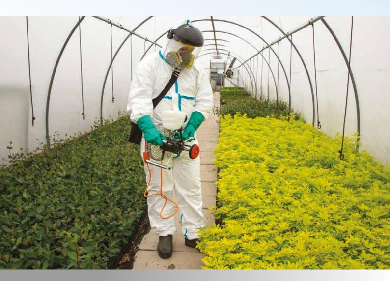
Electrafan is an air-assisted spinning disc sprayer which has been designed for low and ultra-low volume application of insecticides and fungicides in areas with little or no natural air movement.
