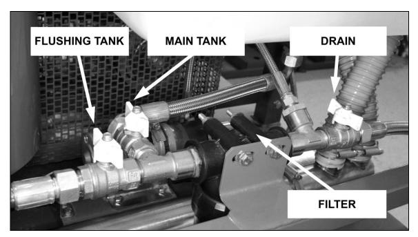
Fig. 2 – Valves & Filter Under Tank
