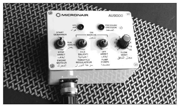
Fig. 1 – Control Box in Cab of Vehicle
