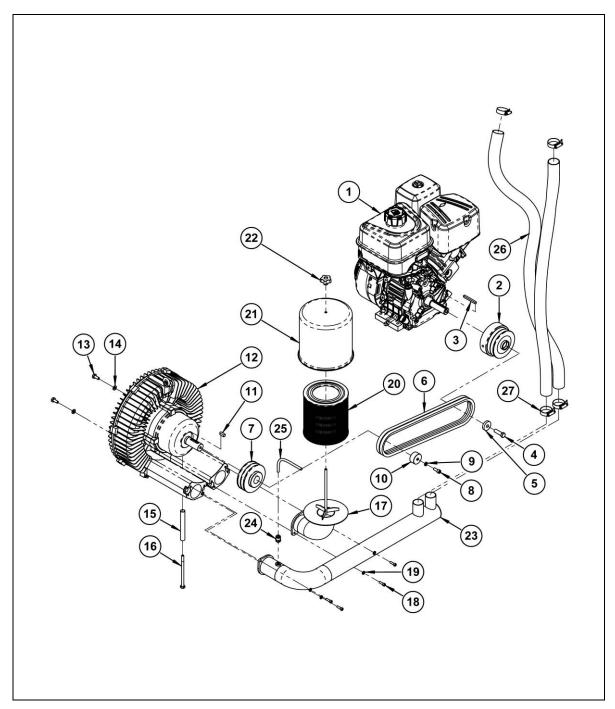
Fig. 13 – Engine, Blower, Drive Belts & Air Tubes
