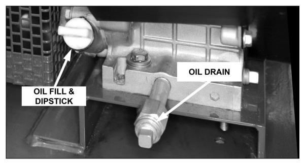
Fig. 6 – Engine Oil Filler and Drain
