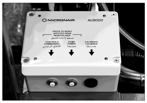
Fig. 4 – Calibration Switch on Junction Box
