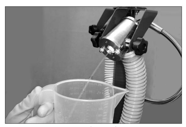
Fig. 5 – Flow Calibration Check
