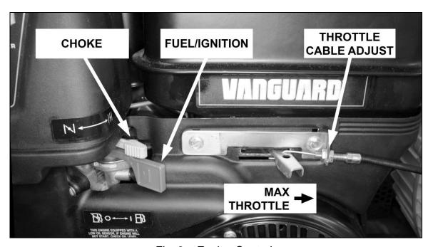
Fig. 3 – Engine Controls
