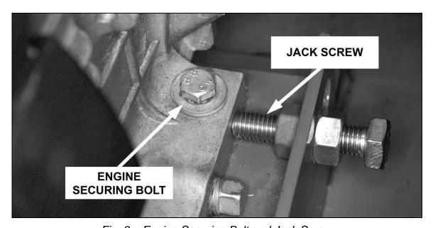
Fig. 8 – Engine Securing Bolt and Jack Screw
