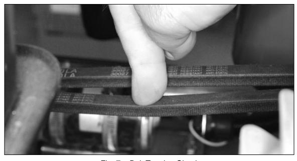
Fig. 7 – Belt Tension Check
