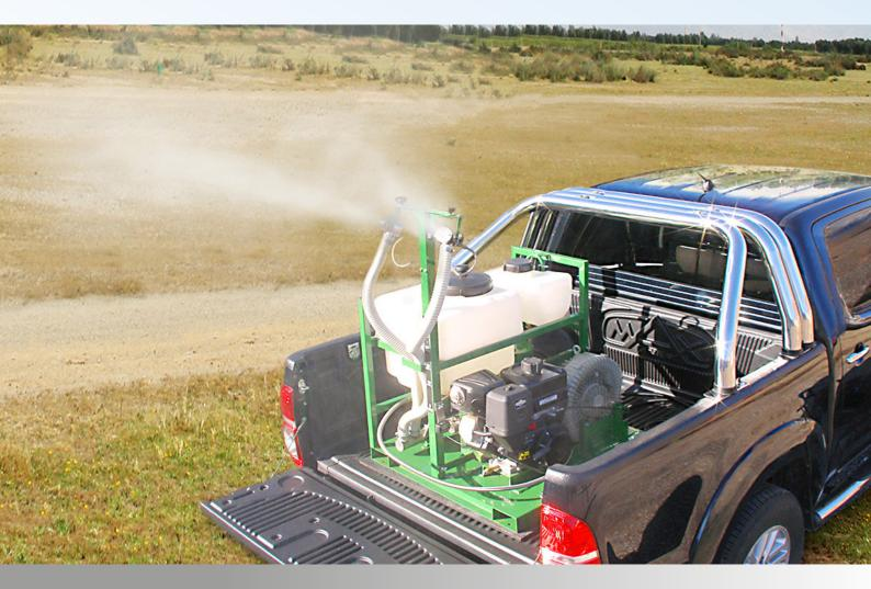
The Micron AU9000 is a vehicle-mounted cold fogger for use with both conventional and watermiscible ULV formulations. Uses include the control of adult mosquitoes, flies and similar pests as well as disinfection and odour control.
