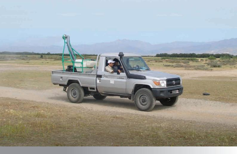
The Micron AU8115MS is a self-contained vehicle-mounted Controlled Droplet Application (CDA) sprayer designed for a wide range of migrant pest, public health and agricultural spraying tasks.
