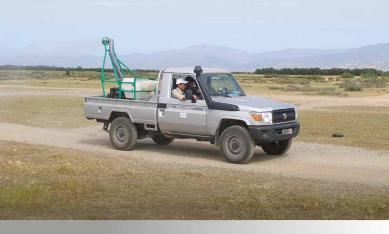
The Micron AU8115 is a self-contained vehiclemounted Controlled Droplet Application (CDA) sprayer designed for a wide range of migrant pest, public health and agricultural spraying tasks.
