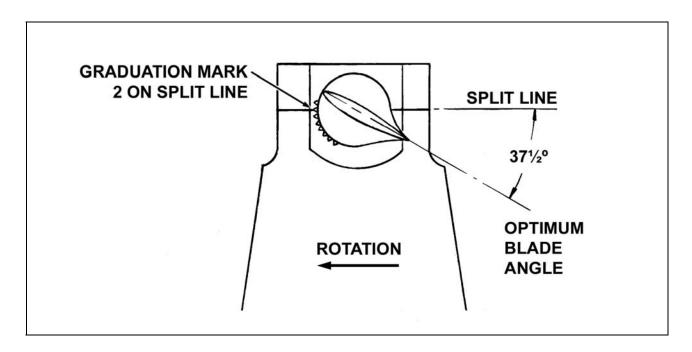
Fig. 4 – Setting Marks on Blade
