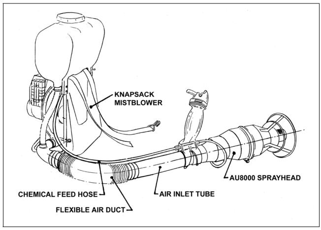
Fig. 1 – Attachment of AU8000 Sprayhead to Mistblower
