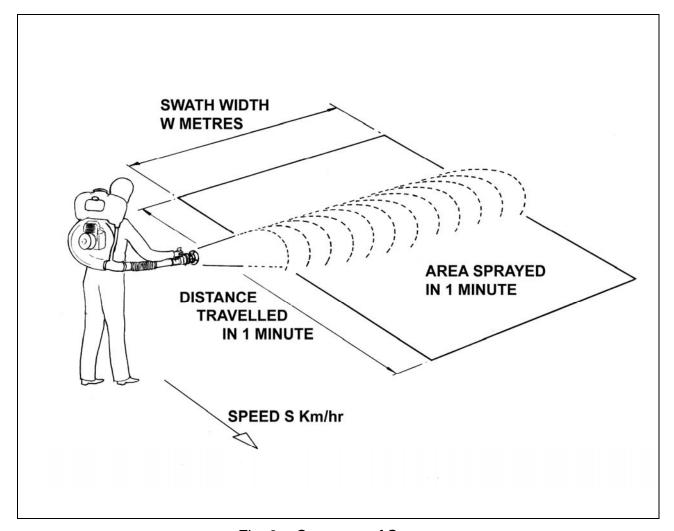
Fig. 3 – Coverage of Sprayer
