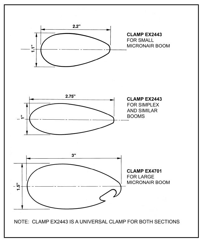
Fig. 3 – Dimensions of Clamps for Streamline Booms
