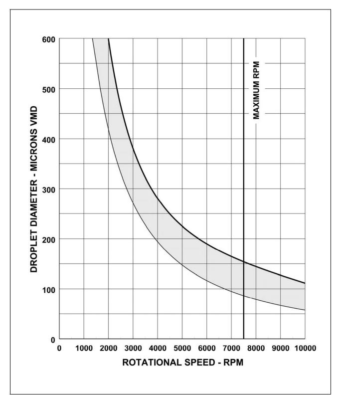
Graph 3 – Relationship Between Droplet Size and Atomiser RPM
