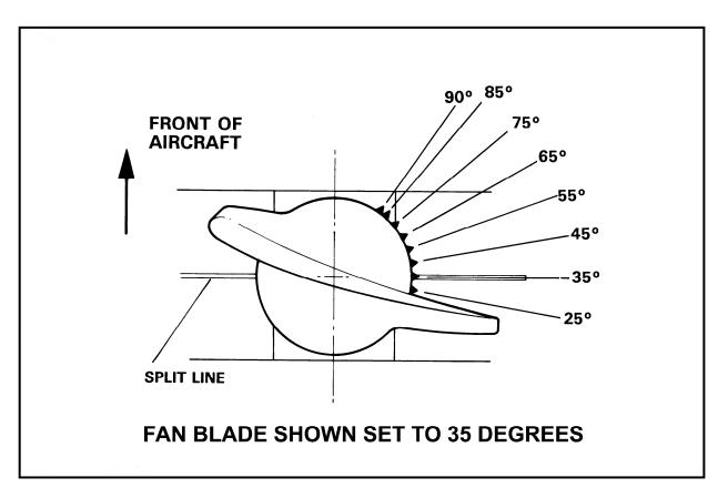
Fig. 6 – Adjustment of Fan Blade Angle
