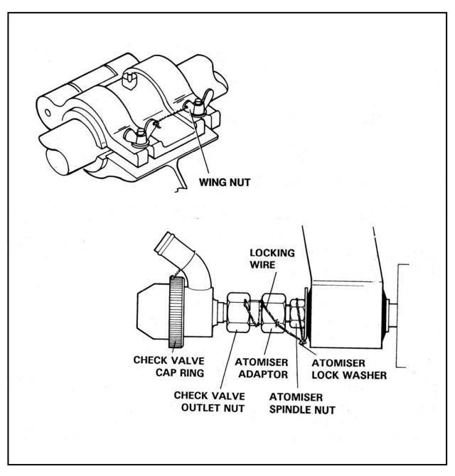
Fig. 2 – Wire Locking of Atomiser and Components
