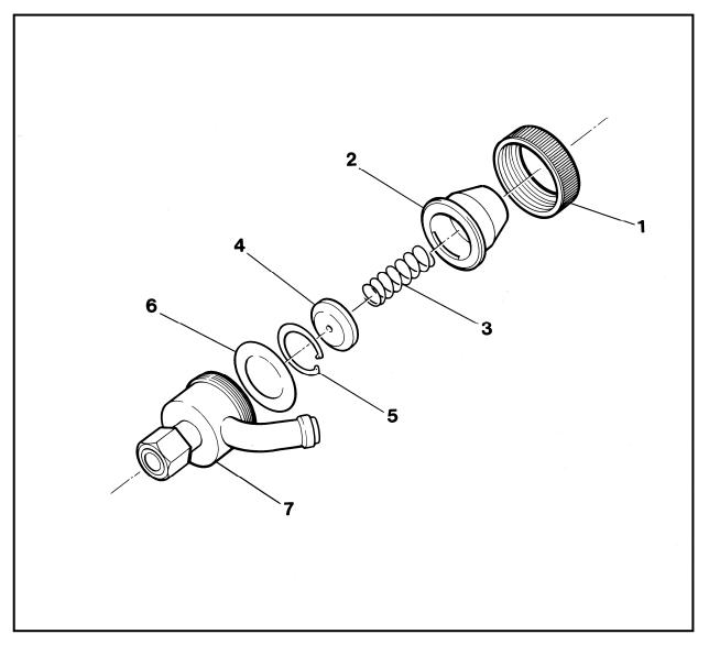
Fig. 10 – Diaphragm Check Valve
