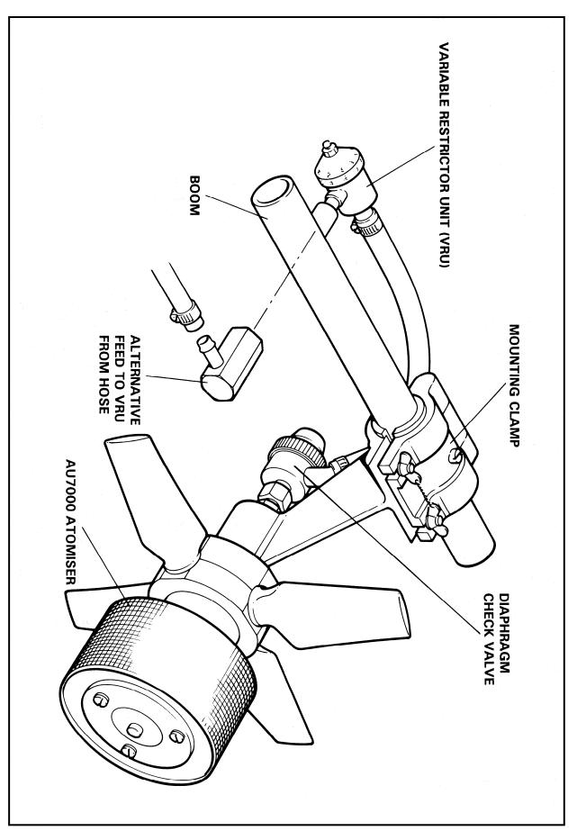
Fig. 1 – Typical Installation of AU7000 Atomiser
