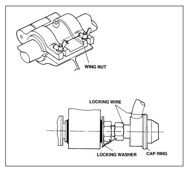
Fig. 2 – Wire Locking of Atomiser and Components
