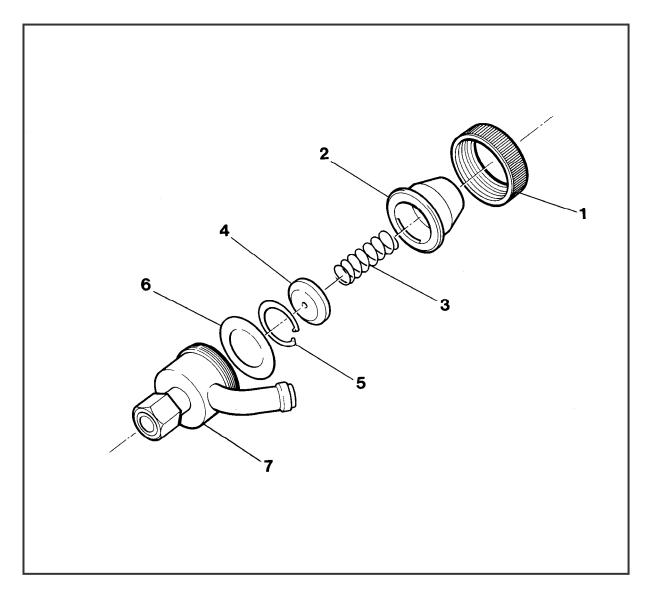
Fig. 11 – Diaphragm Check Valve
