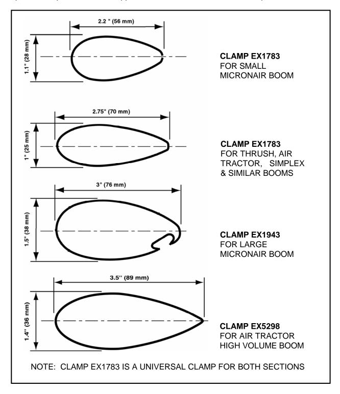
Fig. 3 – Dimensions of Clamps for Streamline Booms
