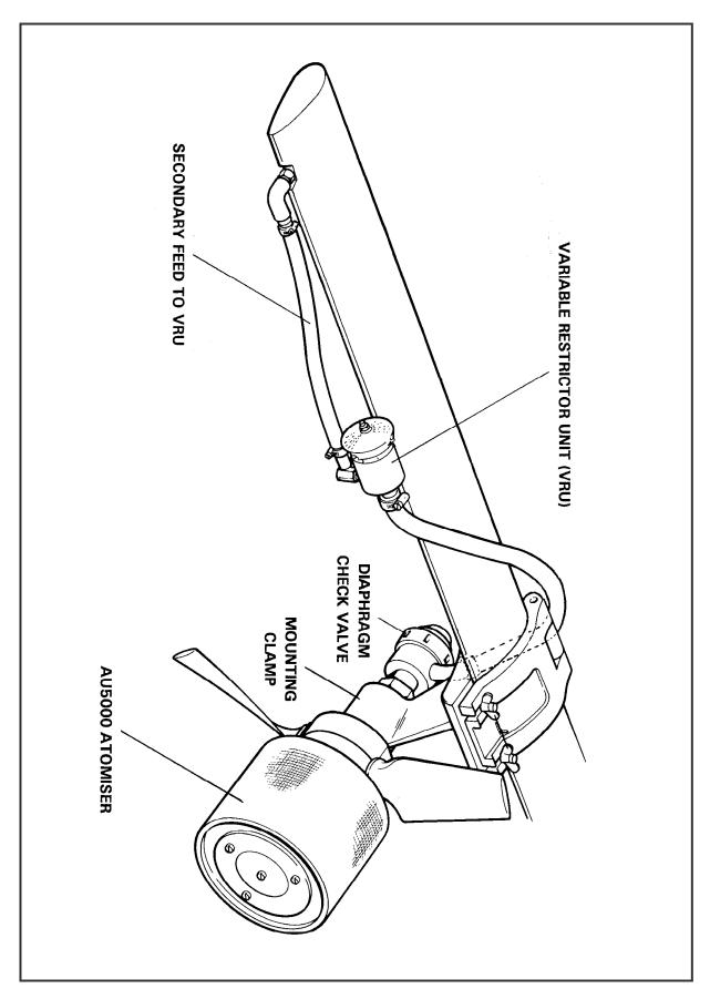
Fig. 1 – Typical Installation of AU5000 Atomiser
