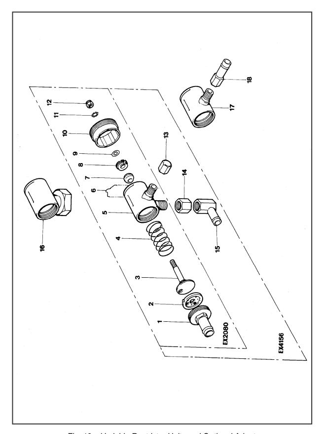
Fig. 10 – Variable Restrictor Units and Optional Adaptors
