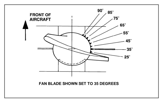
Fig. 5 – Adjustment of Fan Blade Angle
