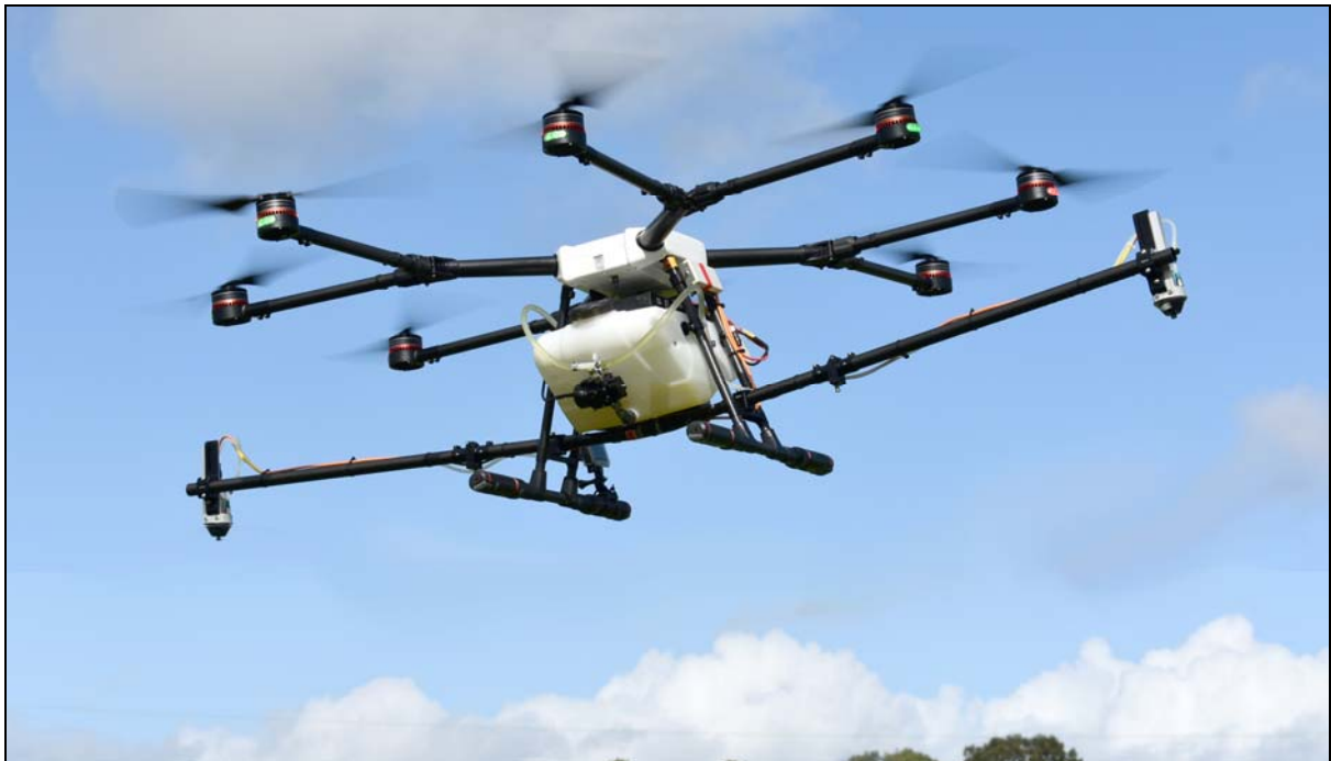
Fig 2. – Micromiser Atomisers on Multi-rotor UAV
